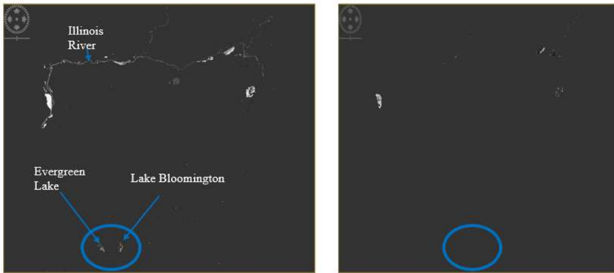
Figure 10. MCI images showing Lake Bloomington and Evergreen Lake (a) September 23, 2018 image (b) August 19, 2019 image. White color indicates areas covered with water while black indicates areas without water.
