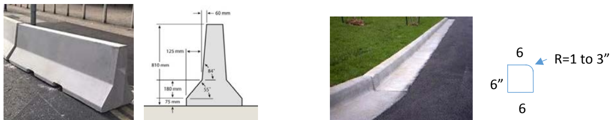
Fig. 7. Standard dimensions F-shaped concrete divider (left) curb (right).
