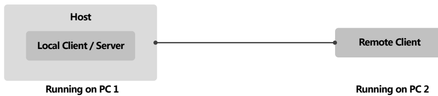
Figure 3.1: The diagram shows the framework of networking of LeMo, i.e. a remote client running on PC2 connects to a host running on PC1.
