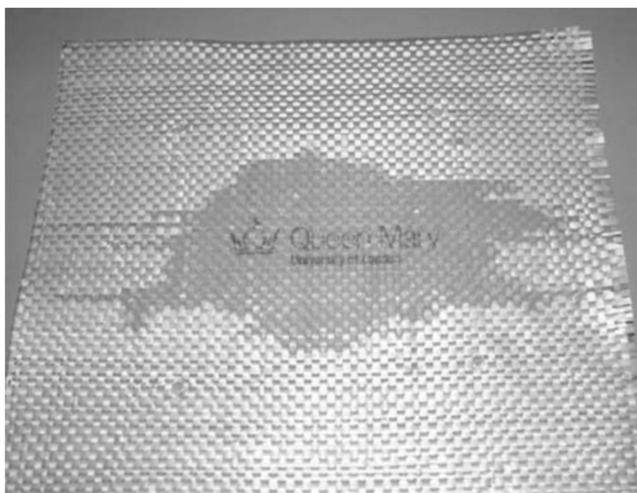
Figure 2.9 Oil absorption by woven all-PP tapes 82 . The originally opaque tapes become semi-transparent when in contact with a small amount of oil in the centre of the fabric.
