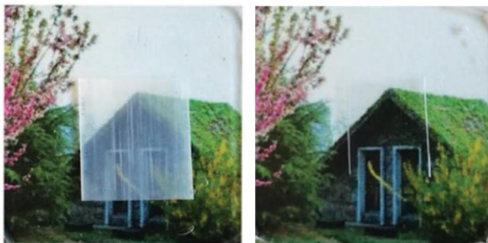
Figure 2.7 Appearance of UHMWPE/graphene (left) and UHMWPE/graphene/BZT (right) nanocomposite films 78 .
