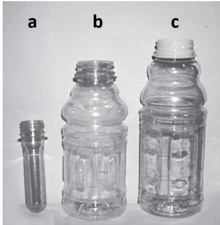
Figure 2.5 (a) PET preform for stretch-blow moulding process, (b) heat-set PET bottle with standard transparent thread and (c) heat-set PET bottle with post-crystallized opaque thread acquired by annealing 64 .
