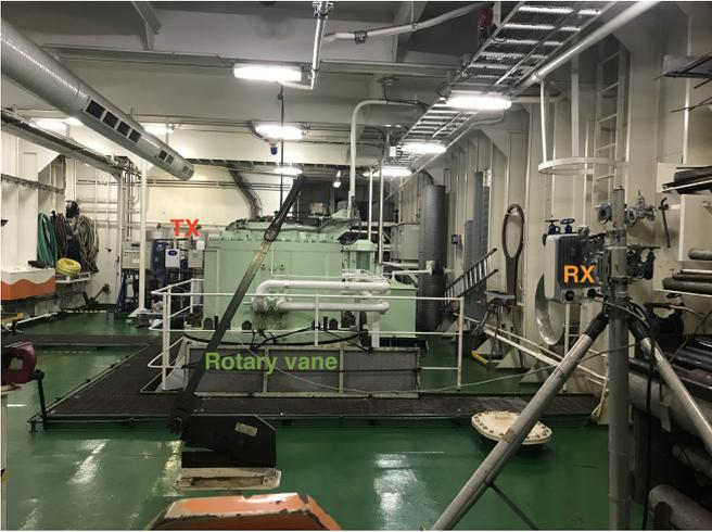
(b) Picture of steering room where the rotary vane is obstructing LOS path between TX and RX
