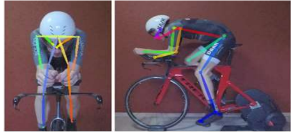
Figure 3: Rider skeleton detection (lab set-up).
