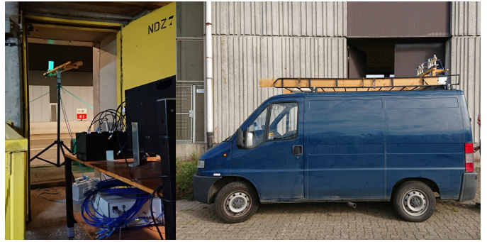
Fig. 2. Tx as a roadside unit with the antenna fixed inside the tunnel through an emergency exit (left) and the van loaded with Rx and the antenna mounted on the rooftop (right)
