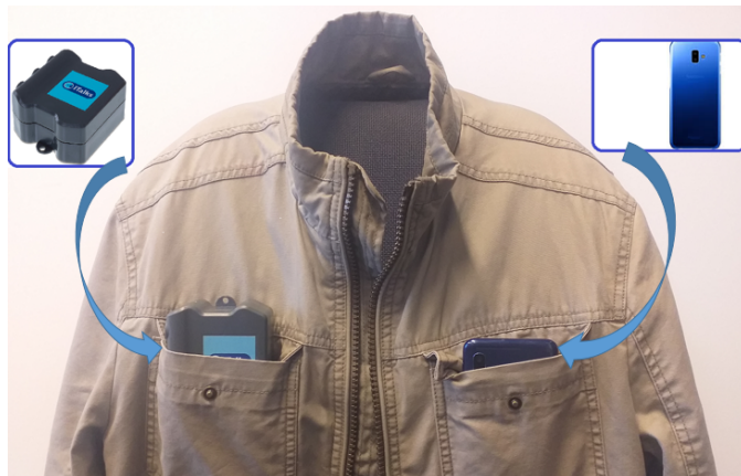
Figure 1: Measurement setup carried within a jacket: Left: TX LoRaWAN node for which we estimate its location. Right: Smartphone which logs the GPS ground truth
