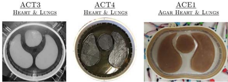
Figure 1. Experimental setups for test phantoms from the ACT3, ACT4, and ACE1 EIT systems.
