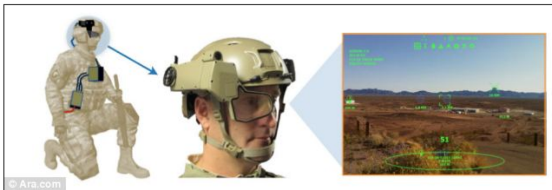
Figure 9. The system is connected to control units on the soldier's body. Information is sent wirelessly to the soldier and displayed over one of their eyes (Prigg, 2014). (Image: https://www.ara.com/national-security )
