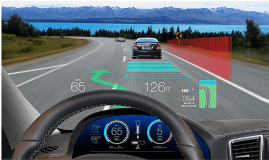
Figure 10. HUD with Texas Instrument DLP technology assists with directions, safety and other information for the driver of the vehicle. (Image: http://www.ti.com/ww/en/dlp/automotive/hud.html?DCMP=HUD&HQS=dlpHUD )
