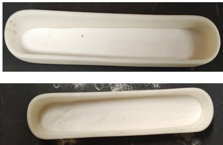
Figure 16. (Top) The fresh boehmite powder before calcination treatment at 550 C. (Bottom) The calcined boehmite powder, while it seems more yellow in the photo, is due to ambient light.
