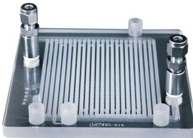
Figure 1. A typical microchannel reactor that is etched into a stainless steel and glass apparatus (Amarequip, 2020).
