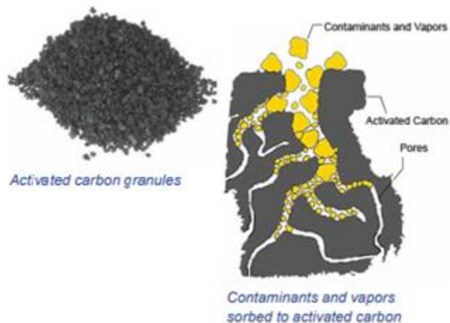
Figure 4: Activated Carbon Schematic (adapted from EPA, 2012)
