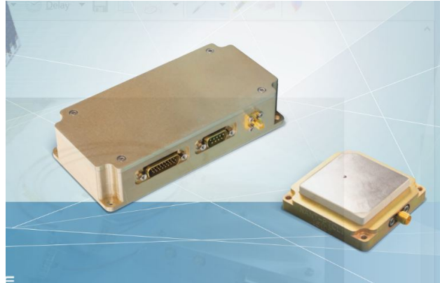
Figure 5: GPS Module and Antenna.
