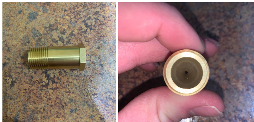
Figure 61: Machined Tapered Nozzle - Right: View of Internal Taper
