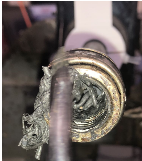
Figure 12: Cleaning a Clog from the Filastruder
