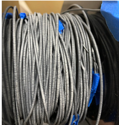
Figure 36: 1 Spool of Iron and PLA (Note the inconsistent diameters)
