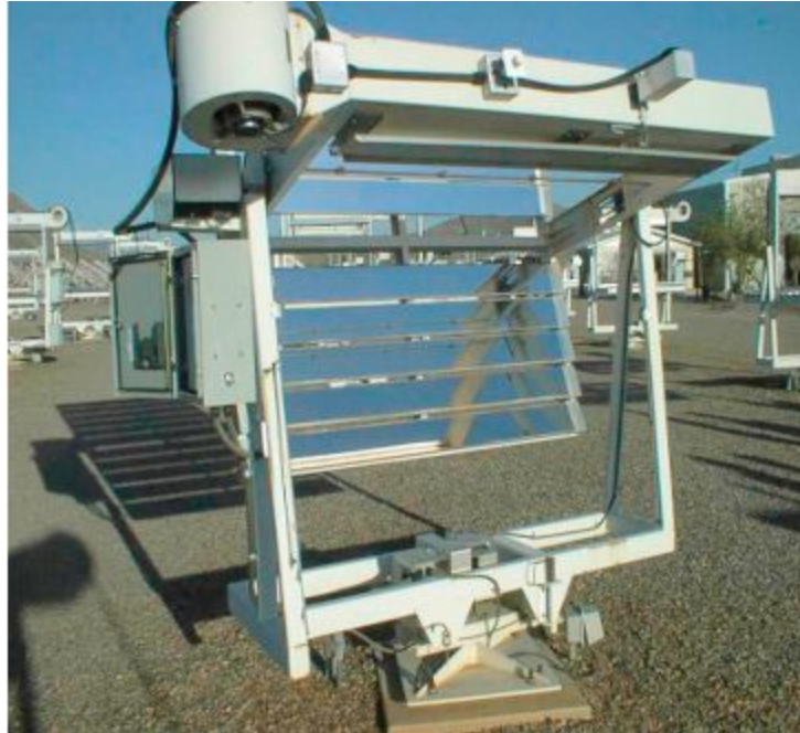
Figure 4: A Solar Fresnel Mirror apparatus in Arizona.
