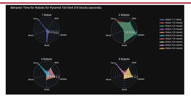
Here is a comparison of different sized swarms working to build a pyramid made of 316 blocks.
