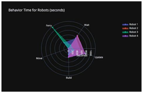
Notice for four robots how the robots spend time working on different tasks, showing interesting characteristics of task specialization and can be used as an area for future research.
