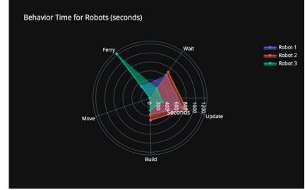
As more robots are added, robots spend time working on (specializing in) different tasks. Some robots spend more time ferrying, while others spend more time building.
