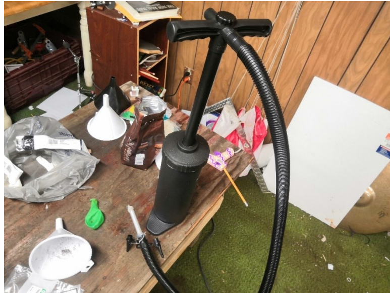
Figure 96: Second Air Pressure Source
