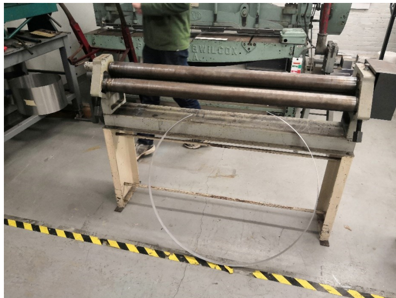
Figure 88: Roll Bending of Track Ring Aluminum Sidewall
