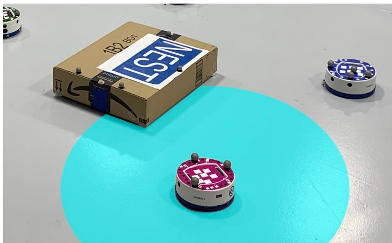
Figure 3.5: Mock up of proximity sensor display
