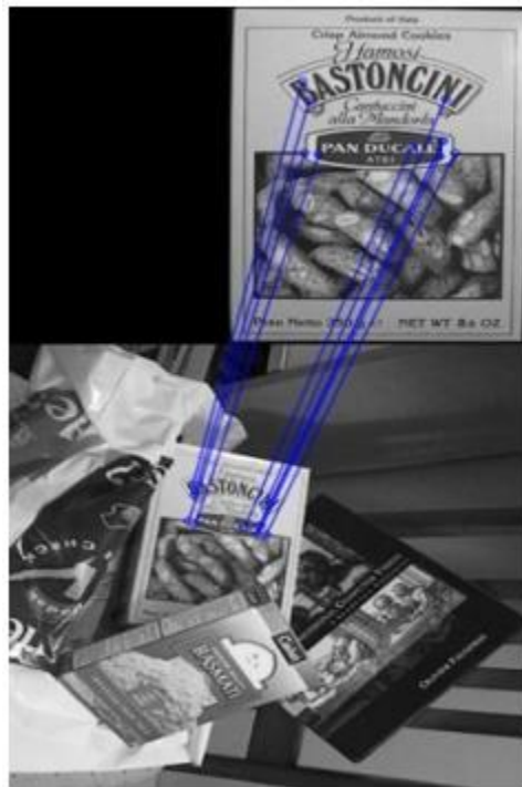
Figure 20. Feature matching example (right) from “OpenCV: Feature Matching”, https://docs.opencv.org/3.4/dc/dc3/tutorial_py_matcher.html
