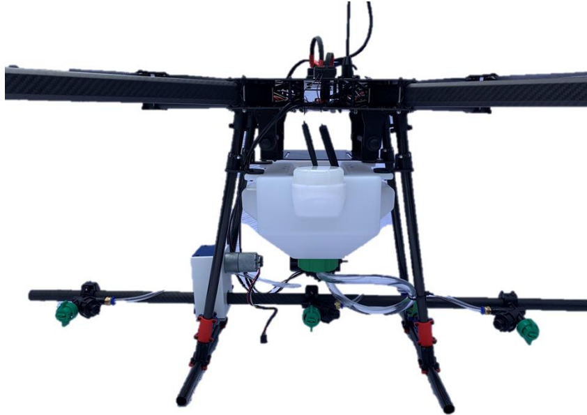
Figure 24. Close-up of spray-bar on the built drone
