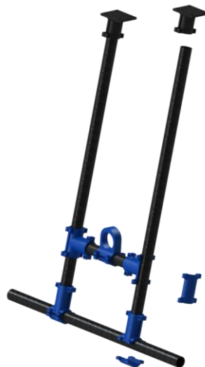
Figure 6. SolidWorks model of drone's landing gear assembly
