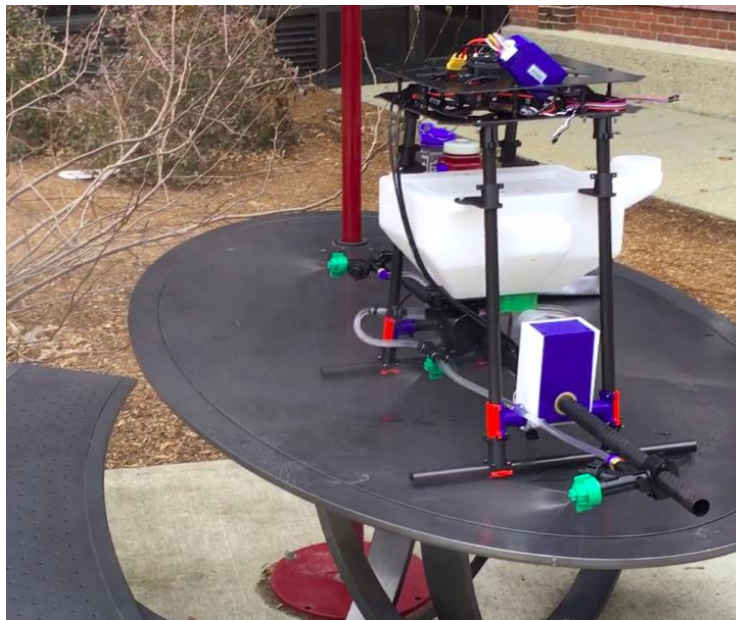
Figure 26. Remote test of three sprayers operating simultaneously
