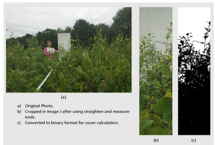
Figure 2: Example of original, cropped and binary photos used for an automated calculation of the percent of the cover board obscured by vegetation.
