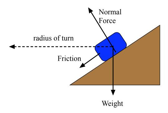
FIGURE 7.2: Sketch of object on a banked curve
