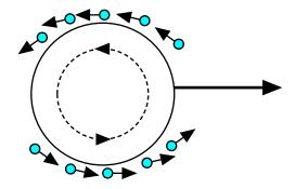
FIGURE 8.16: Sketch of spinning golf ball in flight
