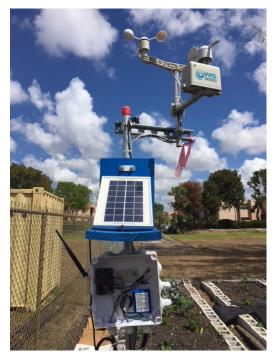
Figure 5.4: WSU connected to a weather station
