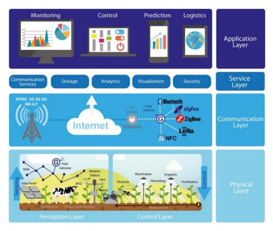
Figure 4.1: IoT architecture in precision agriculture application [5]
