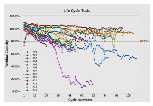
Figure 6.5: Residual capacity against cycle number
