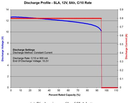
(a) Discharging profile of SLA battery
