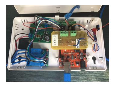
Figure 5.7: The control unit for scheduling irrigation events local or synchronized to an external database. Energy data infrastructure is connected similar to the wireless sensor nodes. The protocol uses Max485 for serial communication between an Arduino Mega and the power meters. Arduino sends voltage, current and power data in frames to router with ZigBee protocol as shown in Fig.5.8.
