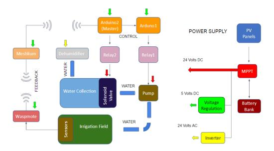
Figure 6.1: Off-grid PV supported integrated FEW system schematic
