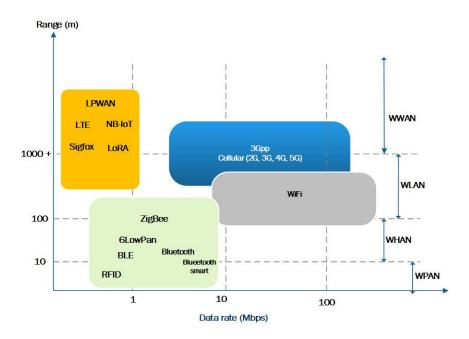
Figure 4.2: Data rate vs. range capacity of wireless communication technologies
