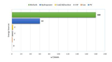
Figure 3.4: Water use by various energy source in electricity production [3]
