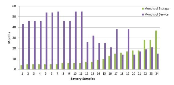
Figure 6.3: SLA battery service span against storage time
