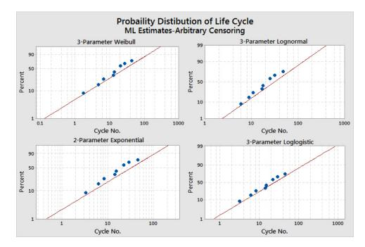
Figure 6.6: Probability Distribution plot of life cycles data of SLA Estimation
