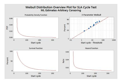
Figure 6.8: Weibull distribution overview plot of life cycle data for SLA battery
