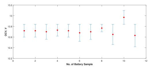
Figure 6.2: Measured OCV of new batteries
