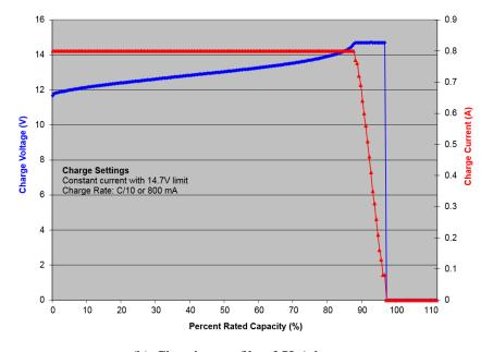
Charge Profile - SLA, 12V, 8Ah, C/10 Rate
