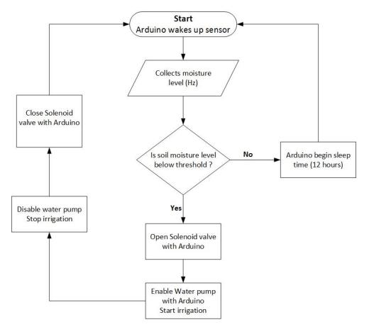
Figure 5.6: Flow chart for control system algorithm
