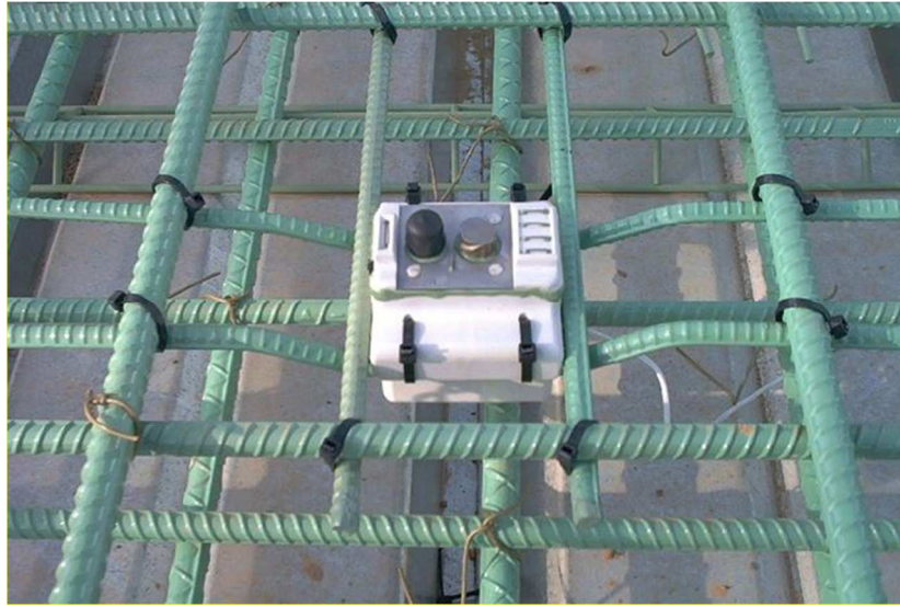
Figure 2-14: Model of ECI-2 Embedded Corrosion Instrument [22]
