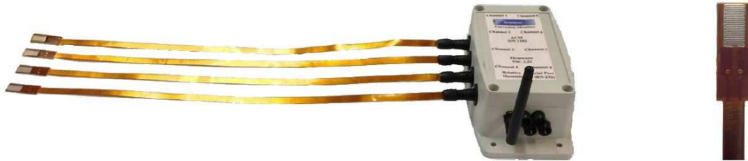
Figure 2-25: Four micro linear polarization resistance ( \mu LPR) sensor with one node (left) and the close-up image of \mu LPR sensor (right) [27]
