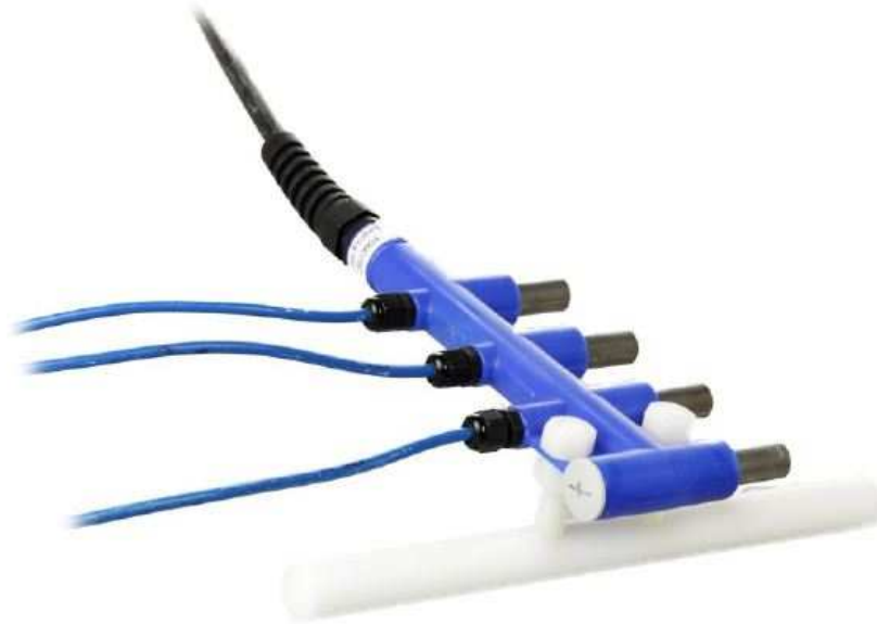
Figure 2-38: M4 corrosion probe configuration [36]
