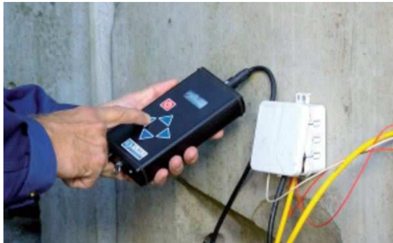
Figure 2-21: Data logging system to measure corrosion current [26]
