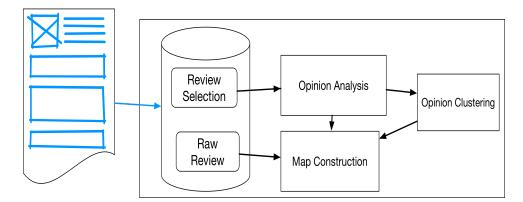
Figure 4.1: System Architecture
