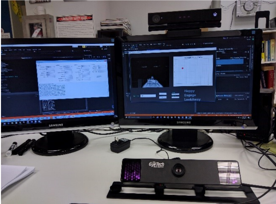
Figure 4.1: An entire system including Kinect V2 (on top of the screen) and TM3 (in front of the computer)
