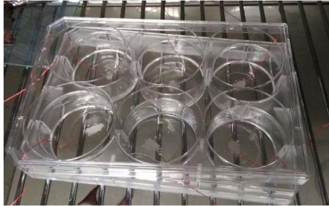
Fig. 3.7 Well plate with electrodes at the bottom coated with hydrogel
