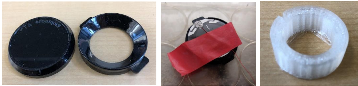
Fig. 3.11 (a) Delta T culture dish (b) Wire attached to the bottom part of culture dish (c) 3D printed top electrode support
