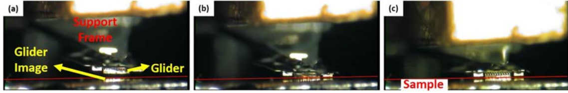
Fig. 10.9 Optical images of the probe as it approaches the sample at room temperature: (a) when Z = 1900\mu m and probe is away from the sample. (b) when Z = 2200\mu m and the probe is barely touching the sample. (c) when Z = 2600\mu m and the probe is laying flat on the sample. In these pictures one is looking from the location denoted with an eye icon in Fig. 10.4.
