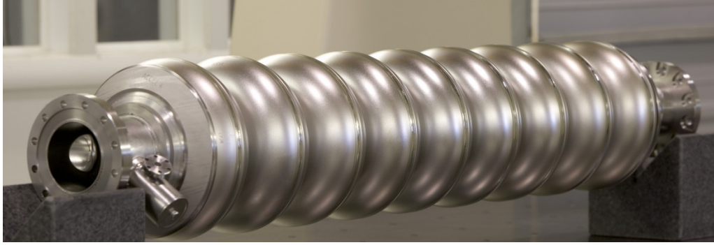
Fig. 2.1 A superconducting TESLA cavity made from bulk Nb. Source: Fermilab ILC–SRF R&D webpage [49].
