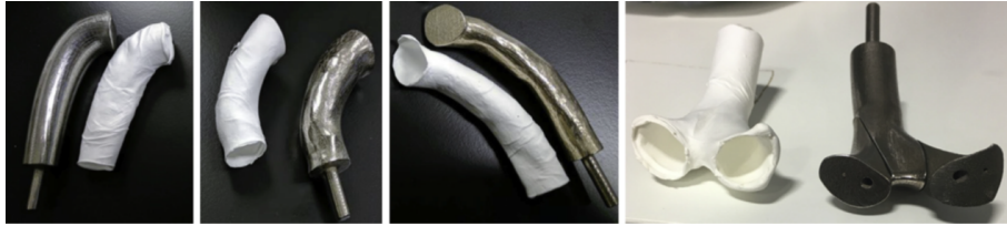
Figure 1.8: Pairs of 3-dimensional printed mandrels and electrospun biodegradable grafts. Reprinted from The Journal of Thoracic and Cardiovascular Surgery , Siallagan, D. et al., Virtual surgical planning, flow simulation, and 3-dimensional electrospinning of patient-specific grafts to optimize Fontan hemodynamics, 155(4):1743-1742, 2018, with permission from Elsevier.
