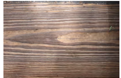
Figure 1ad. Wood2: Close-up of unpainted wood floor with eroded, darkened surface closely following wood grain.
