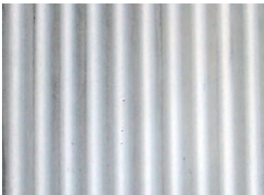
Figure 1v. Metal3: New corrugated steel sheet.
