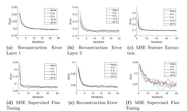
**Figure 4.14:** Progress of training with RBMs as hidden layers for (a)-(d) MNIST dataset, with 2 hidden layers each of 200 units, and (e)-(f) WBCD dataset, 1 hidden layer with 40 units. (a) and (b) show the reconstruction error on the  $1^{st}$  and  $2^{nd}$  layers respectively. (c) and (d) are the classification Mean Square Error with FE and SFT.
