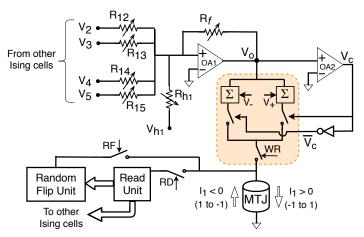
Figure 5.4: The proposed Ising spin cell. Switches WR, RD and RF are turned on in the Write, Read and Random Flip stages respectively.
