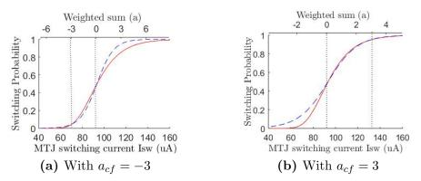
**Figure 4.11:** Switching probabilities of the MTJ (solid red line) meant to store RBM hidden unit's states as a function of  $I_{sw}$ , and desired hidden unit's activations as output of sigmoid (dashed blue line) for (a)  $a_{cf} = -3$ , and (b)  $a_{cf} = 3$ . Vertical dashed lines in the plots depict the matching at respective values of  $a_{cf}$ . In (a), the parameters are  $I_0 = 93.28\mu A$ ,  $I_{cf} = 70.38\mu A$ . Maximum read voltage  $V_{rd} = 0.2 V$  has been used throughout.
