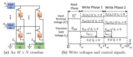
Figure 4.4: The 1T1R crossbar. (a) Schematic (b) Read & write phases signals
