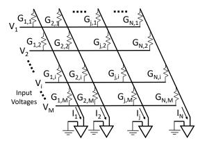
Figure 2.5: Structure of an  $M \times N$  resistive crossbar
