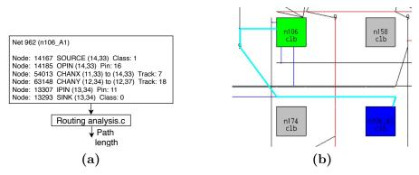
Figure 5.8: Routing of nets. (a) The source, sink and path of a net in textual form in the *.route* file. (b) View of the routing. The source is in dark blue and the sink is in green. The net has been highlighted by us in sky blue.
