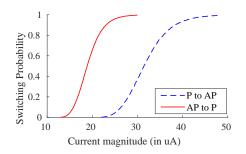
Figure 5.2: Switching probabilities of the MTJ with 2ns pulse width. Note that current polarities would be opposite for  $P \rightarrow AP$  and  $AP \rightarrow P$ . Data obtained from MTJ Stochastic LLG simulations [37, 6] in HSPICE, at steps of  $0.1\mu A$  with 10000 points per step.
