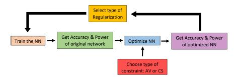
Figure 3.6: Flow chart showing the process and network optimization and characterization. We start with training an NN without regularization.
