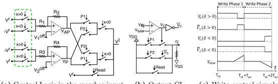
(a) Control Logic in the crossbar input (b) Output CL (c) Write control signals terminals.
