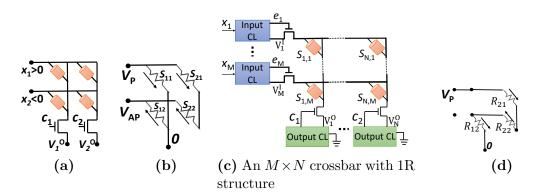
**Figure 4.6:** (a) and (b) Alternate current paths in the 1R structure with 2-phase write strategy - (a) A 2 × 2 crossbar. (b) Its equivalent circuit in write phase 1 with  $c_1 = V_{DD}, c_2 = 0, V_1^O = 0, V_1^I = V_P, V_2^I = V_{AP}$ . (MTJ synapses shown as resistors). (c) Schematic of the proposed 1R Architecture for MTJ crossbar, (d) The equivalent circuit in phase 1 with 4-phase writing.
