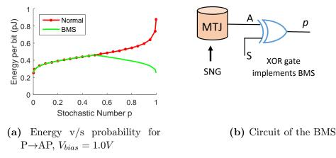
Figure 3.3: (a) Variation of energy with value of SN p with and without BMS (green undotted and red dotted lines respectively). (b) The BMS.
