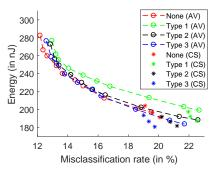
Figure 3.7: Energy vs classification error rate curve for the MNIST dataset 1-layer NN. The dots are for the AV constraint, whereas the asterisks are for CS. Optimization was done with 1000 training samples.
