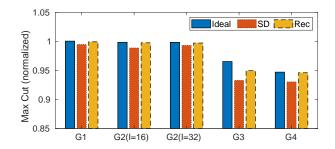
Figure 5.12: Max cut values (normalized) from the Ising simulations for the 4 graphs, with 2 different values of Ising cell fan-in (I) used for G2.
