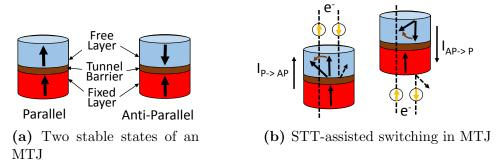
**Figure 2.3:** (a) The MTJ (b) Spin-Torque Transfer switching from  $P \rightarrow AP$  (left) and  $AP \rightarrow P$  (right). Dashed lines show the path of oppositely spin-polarized electrons.
