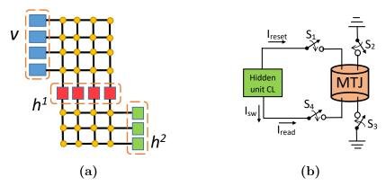
**Figure 4.10:** (a) DBN crossbar structure -  $4 \times 4$  and  $4 \times 3$  crossbars for the  $1^{st}$  and  $2^{nd}$  hidden layers. (b) Circuit of MTJ as RBM hidden unit connected to the respective Control Logic.
