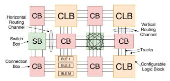
Figure 5.6: The FPGA architecture. CLBs are connected through CBs and SBs.
