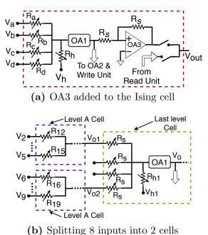
Figure 5.5: (a) The Modified Ising cell. (b) Multi-level Ising cells. Observe that
