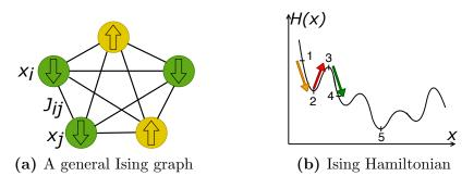
Figure 5.1: (a) An Ising graph with 5 spin units. (b) The system transitions from state 1 to 2, a local minima. Random perturbations can take it to state 3 so that it transitions to 4 and can eventually reach global optimum 5.
