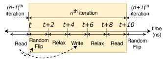
Figure 5.3: Different stages of an iteration in the process of finding the ground state of an Ising model. Each stage is of duration 2ns, and hence an iteration takes 10ns. The dashed arrows show where the spin value read is utilized.
