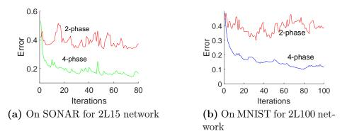
Figure 4.13: Comparison of error during training of the 1R crossbar with 2-phase and 4-phase update schemes for 2 datasets. No variations assumed.
