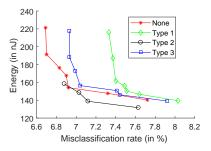
Figure 3.8: Plot of classification error rate against energy for 2-layer NN of MNIST dataset with AV constraint.
