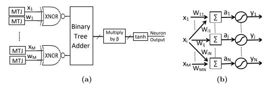
Figure 3.4: (a) Neuron implementation in ISC. The outputs of the binary tree adder and multiplier consist of multiple bit-streams. (b) Schematic of 1-layer NN
