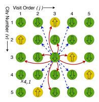
Figure 5.10: Arrangement of Ising spin units for a 5-city TSP. Arrows show interactions of  $x_{3,3}$  - solid red ones enforce constraints, whereas dashed blue ones promote progress of tour.
