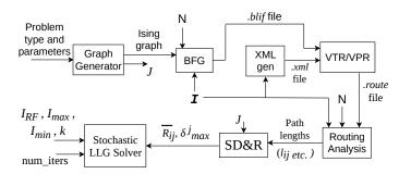
Figure 5.11: Steps performed in the simulations. We start with the Graph Generator and end with the Stochastic LLG simulations.
