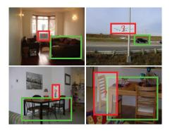
Figure 5.6: **SCN contextual classification.** Features of the top stream (red boxes) are predicted using patches from bottom stream (green boxes) and offset vector as inputs to the trained SCN. A classifier is then trained to predict the label of the red patch based on the *predicted* features from the training set. Performance on testing set is 56.3% (Table 5.1).
