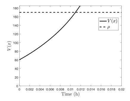
**Figure 17.** V(x) throughout the first sampling period with  $x_1 = 0.2 \text{ kmol/m}^3$  and  $x_2 = 5 \text{ K}$  and  $\rho' = 30$ .
