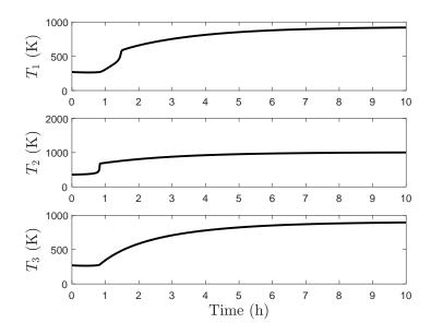
**Figure 5.** *T*<sub>1</sub>, *T*<sub>2</sub>, and *T*<sub>3</sub> over 10 h of operation for the 2 CSTR-flash drum process under a cyberattacked EMPC provided the false state measurement  $x_{F1} = \bar{x}_{u,2}$ .
