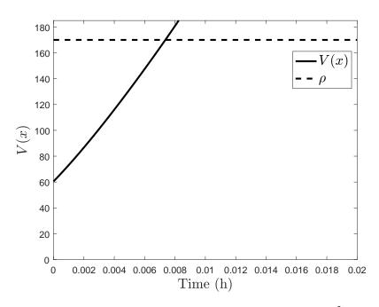
**Figure 16.** V(x) throughout the first sampling period with  $x_1 = 0.2 \text{ kmol/m}^3$  and  $x_2 = 5 \text{ K}$  and  $\rho' = 170$ .
