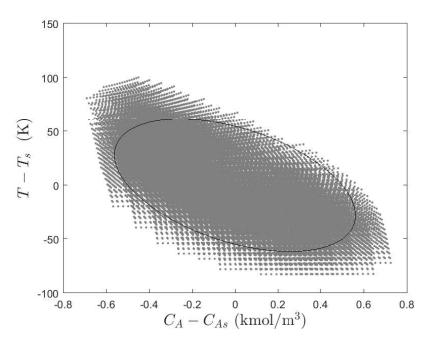
**Figure 8.** Final states after one sampling period when initialized in the stability region and for multiple inputs within the input bounds applied.
