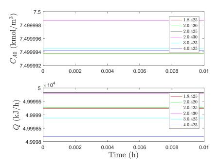
**Figure 12.** Values of  $C_{A0}$  and Q for one sampling period for various cyberattack scenarios.
