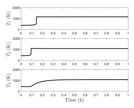
**Figure 3.**  $T_1$ ,  $T_2$ , and  $T_3$  over 1 h of operation for the 2 CSTR-flash drum process under a cyberattacked EMPC provided the false state measurement  $x_{F1} = \bar{x}_u$ .
