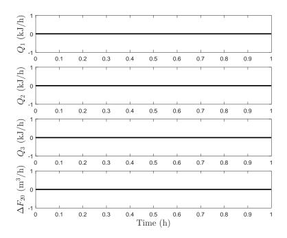
**Figure 4.** Manipulated inputs over 1 h of operation for the 2 CSTR-flash drum process under a cyberattacked EMPC provided the false state measurement  $x_{F1} = \bar{x}_u$ .
