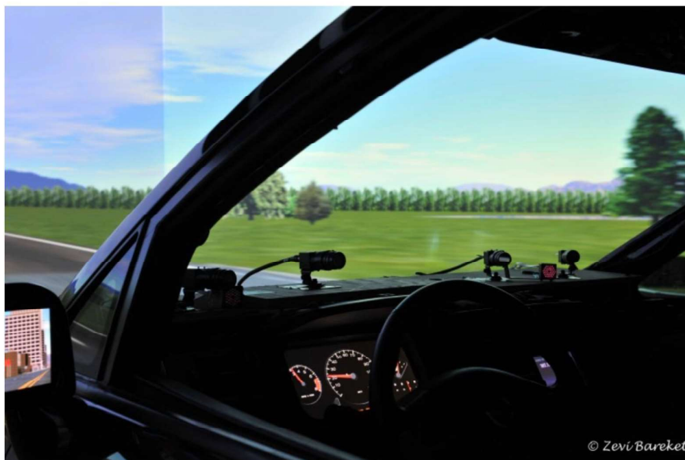
Figure 2. A SmartEye four-camera eye-tracking system in a virtual driving simulator environment ( http://www.umtri.umich.edu/what-we-offer/driving-simulator , accessed on 18 March 2020, with permission given from University of Michigan Transportation Institute (UMTRI) [56].
