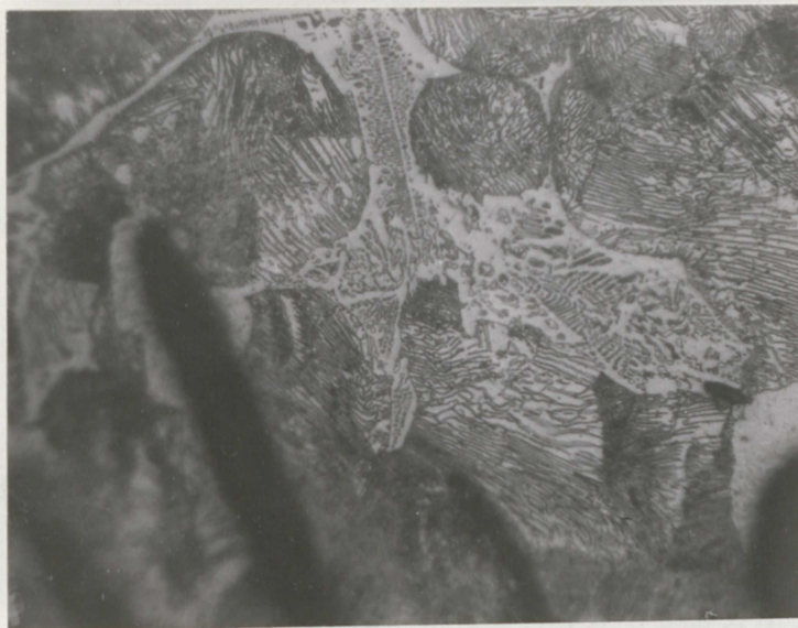
Figure 18 Gray cast iron etched in 4% nital at 450 X under normal illumination.
