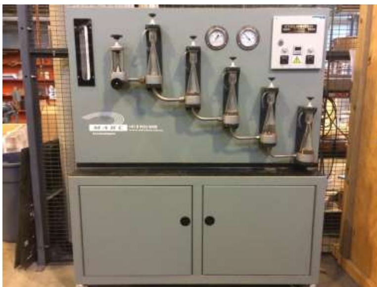
Figure 23: Image of the Warman M16 Hydrocyclosizer
