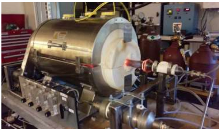
Figure 20: ATS Rotary Furnace Setup for Carburization Experiments
