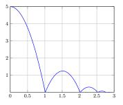
representing the dependency of the ball's hight in time. Among other things, this example demonstrates *Zeno behaviour* which is inherent to hybrid systems: infinitely many iterations occur in finite time.
