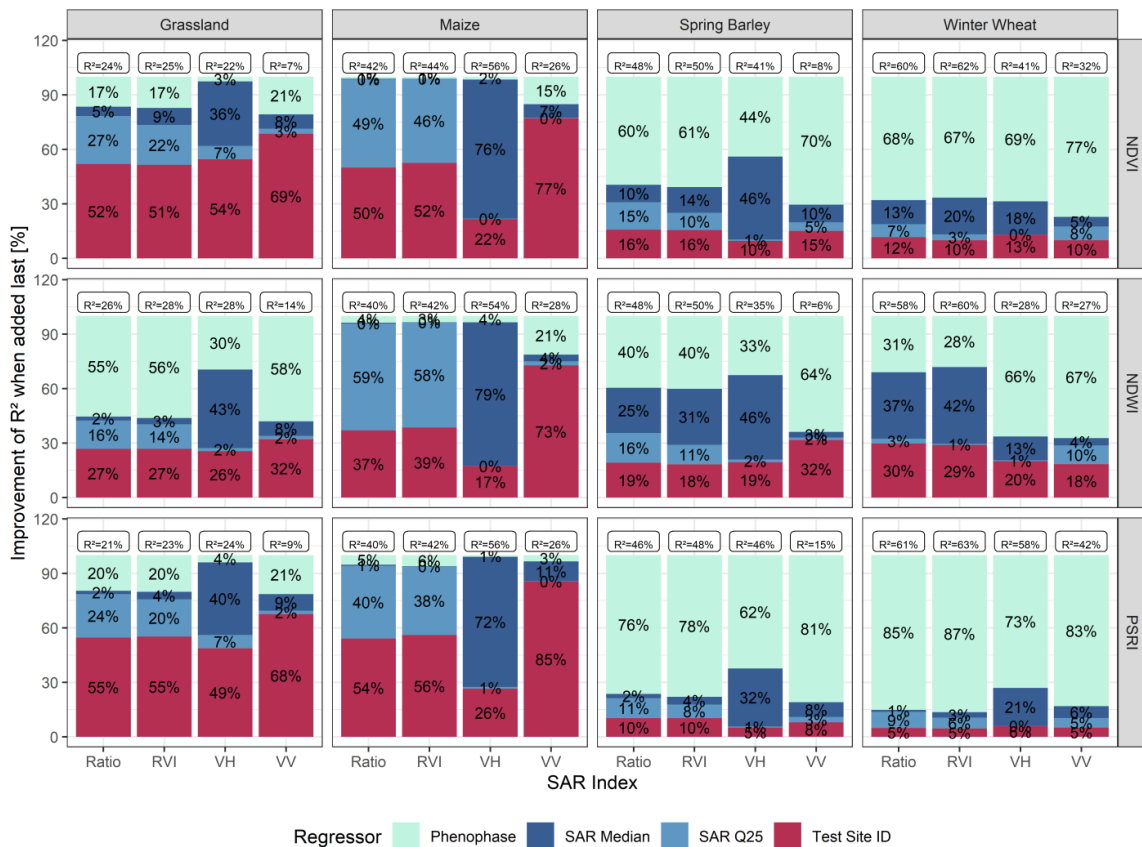
Figure A2. Variable importance of the multiple linear regression analysis for all optical index and SAR index pairs by land use type.
