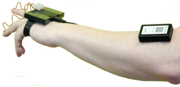
Figure 1: The presented hand sensor system consisting of the base unit , two sensor strips , and one wireless sensor .
