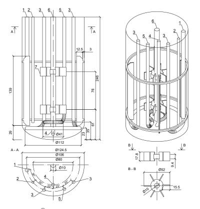
**Figure 1.** Sketch of BioFlo<sup>®</sup> 115 bioreactor: 1—tube for temperature sensor; 2—sampling tube; 3—thermostatic circuits; 4—blowdown connection; 5—sparger; 6—shaft; 7—impeller.
