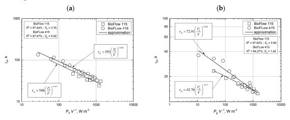
**Figure 9.** Influence of specific power consumption on the mixing time for (**a**) ungassed conditions; (**b**) gassed conditions ( $V_g = 0.083 \,\mathrm{dm}^3 \mathrm{s}^{-1}$ ).
