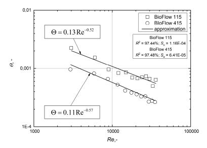
**Figure 7.** Dependence  $\Theta = f$  (Re) for the tested bioreactors.
