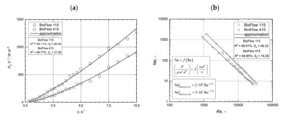
Figure 4. Power consumption per unit volume versus impeller rotational speed (a) and power characteristics (b) for the tested bioreactors.
