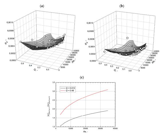
**Figure 8.** The dimensionless mixing number variation with Reynolds number and flow number for: (a) BioFlo<sup>®</sup>115 ( $R^2 = 97.28\%$ ;  $S_e = 2.99 \times 10^{-5}$ ); (b) BioFlo<sup>®</sup>415 ( $R^2 = 95.37\%$ ;  $S_e = 5.31 \times 10^{-5}$ ); (c) comparison of the calculated variation of  $(\Theta_g)\Big|_{BioFlow 115} \Big[(\Theta_g)\Big|_{BioFlow 415}\Big]^{-1}$  with the selected flow number.
