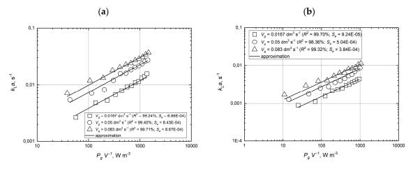
**Figure 12.** The comparison of the volumetric mass transfer coefficient at various gas flow rates for the tested BioFlo<sup>®</sup> 115 (**a**) and BioFlo<sup>®</sup> 415 (**b**) bioreactors.
