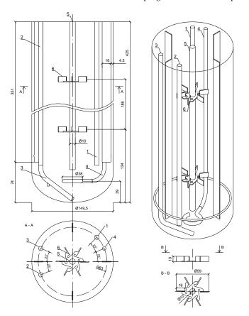
**Figure 2.** Sketch of BioFlo<sup>®</sup> 415 bioreactor: 1—tube for temperature sensor; 2—sampling tube; 3—batching tube; 4—sparger; 5—shaft; 6—impeller.
