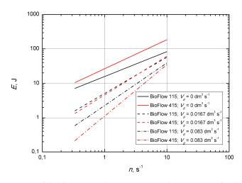
**Figure 10.** The comparison of the dimensional mixing energy characteristics for the tested bioreactors under ungassed and gassed conditions.
