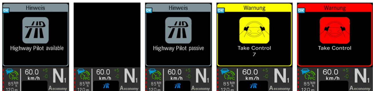
Fig. 2 Automation system warnings in the instrument cluster between speedometer and rev counter. Left to right: (1) automation available and ready for activation. (2) Automation function activated as symbolized through blue 'HP' symbol. (3) Activation function passive
