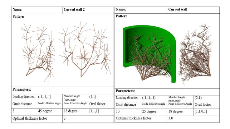
Figure 22 Left: curved wall with omit distance of 8 and equal oval factor. Node effective angle is 45 degree. Right: curved wall with omit distance of 10 and equal oval factor. Node effective angle is 25 degree
