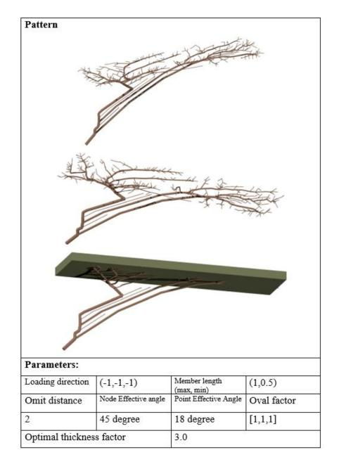
Figure 17 parameters are 45 degree for node effective angle and oval factor of 1 in all three directions
