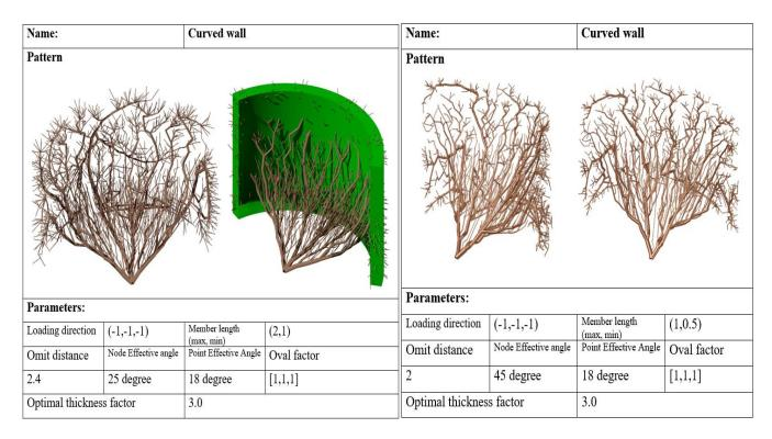
Figure 21 Left: curved wall with omit distance of 2.4 and equal oval factor. Node effective angle is 25 degree. Right: curved wall with omit distance of 2 and equal oval factor node effective angle is 45 degree. The target area portion of a cylindrical shell, which is shown in green color
