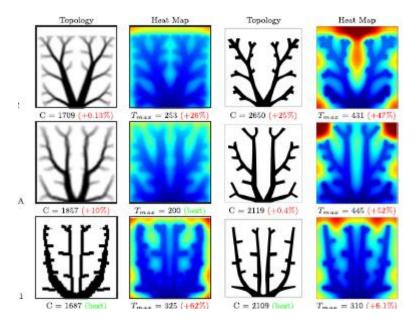
Figure 11 (Lohan et al., 2017) (p.1075), comparison of different heat conducting methods.
