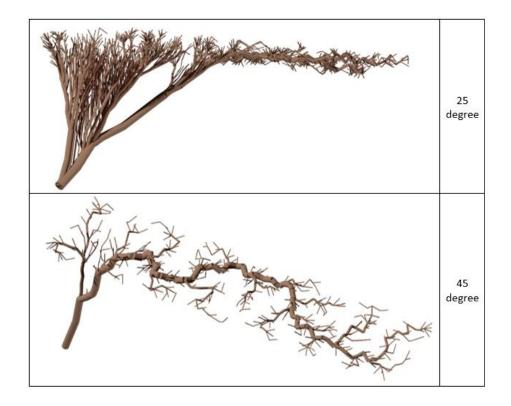
Figure 19 comparison between the 25 and 45 degree approach. In 25 degree the further parts of target area was not covered by nodes in more vertical branches and thus new branches arise with more horizontal inclination
