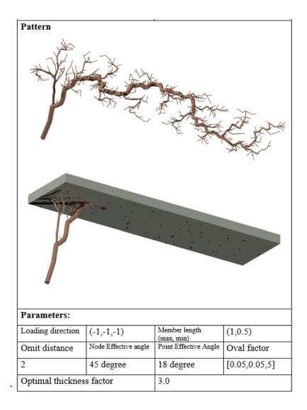
Figure 18 bridge with 45 degree and 0.05 on horizontal and 5 on vertical oval factor
