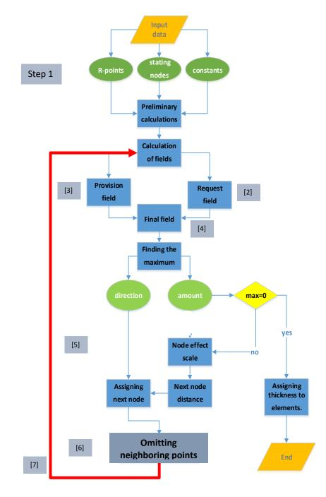
Figure 13 flowchart of pattern generation algorithm
