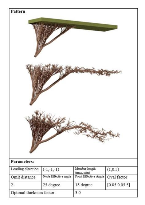
Figure 16 the name 'bridge' is chosen for this shape because of a flat surface that looks similar to a half span of a bridge being supported from bottom. Parameters are 25 degree and 0.05 on horizontal and 5 on vertical oval factor
