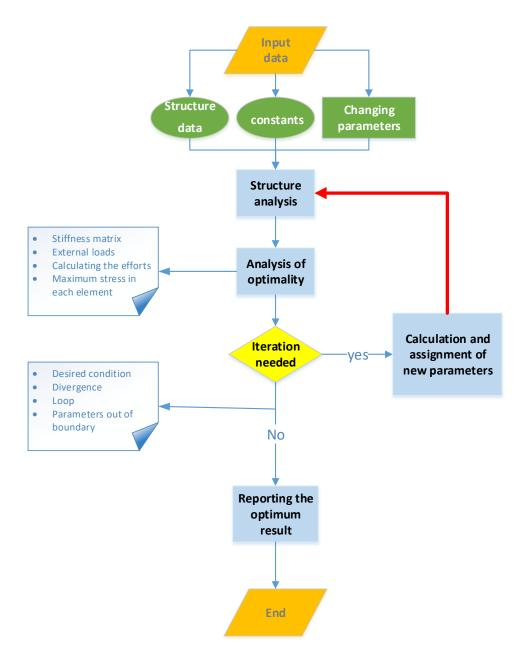
Figure 14 flowchart of structure analysis
