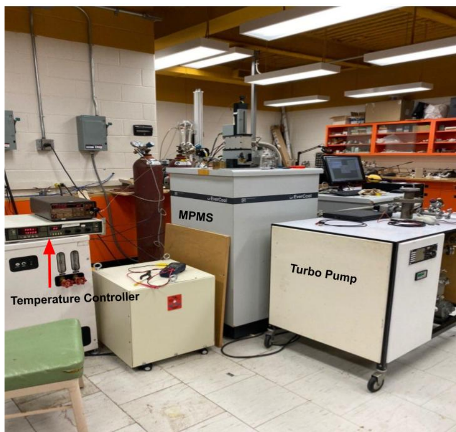
Figure 3.3: On the left the temperature controller is shown, as well as, a volt-meter(middle) to check the furnace temperature using a thermocouple. In front of the system the vacuum pump is seen which is connected to the head block on the MPMS.
