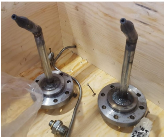
Fig. 9 Injectors used for the lubrication of the upper gearbox transmission components
