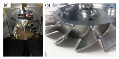
Fig. 1. (a) blisk semi-finish process; (b) finished blisk component.
