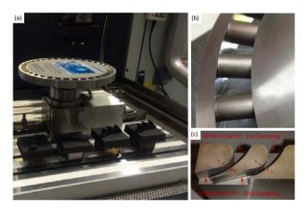
Fig. 4. (a) The whole blisk and the electrodes; (b) cavity image; (c) a previous test in which a cut was made to measure.
