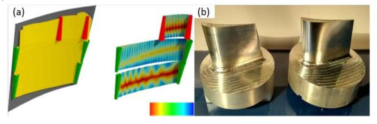
Fig. 2. (a) tool axis motion and color-coded approximation; (b) manufactured blisk blades
