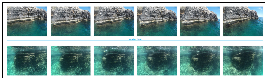
Figure 5. A set of time-lapse images collected awl and bwl at site 2 (Premantura, Croatia). Overlap exceeds 90% at the aforementioned selected swimming speeds. The system is mainly intended for corridor mapping along the waterline with a single strip. If needed, a camera inside the dome in the bow, shown in Figure 6A,C,D, at the water level can be used to film the survey operations.
