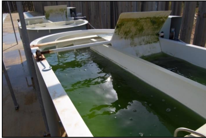
Figure 1.2. Cyanobacterial cultures in open raceway systems. The picture shows a raceway pond with paddle wheel. The main advantages of open systems are their low cost and ease of construction and operation.
