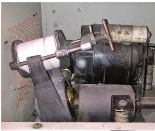
Figure 1.6: YSZ bowl in the Spex8000 shaker mill.
