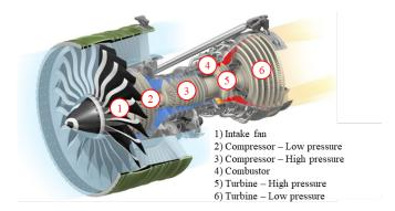
Figure 1.3: Major sections of a gas turbine engine (GE90-series)
