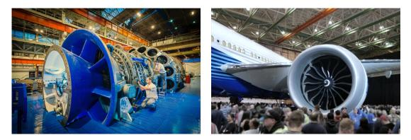
Figure 1.2: Gas Turbines of General Electric: HArriet, heavy-duty gas turbine (left side) and the new Boeing 777X will feature GE9X engine (right side)
