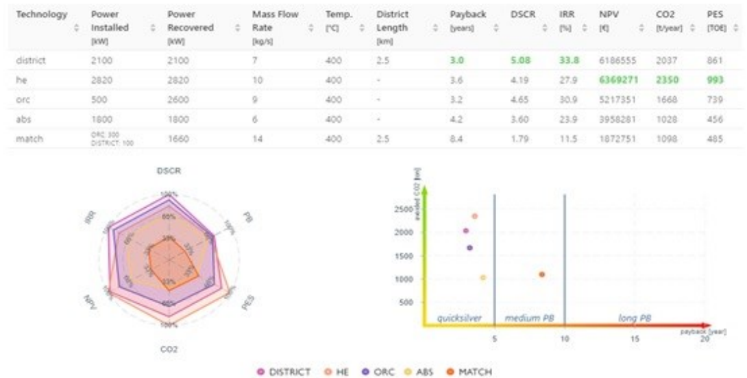
Figure 7.2 CE-HEAT DSS toolbox’s user interface: comparison between different waste heat recovery options (Ciotti et al., 2019).
