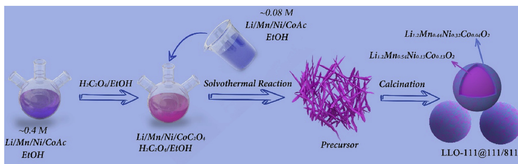
Fig. 1. Schematic illustration for the synthesis of LLO-111@111/811 cathode material.
